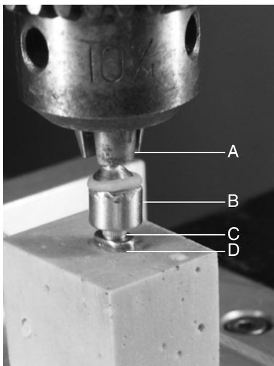
**Fig. 3.** A one-tooth (implant) model was used to evaluate retention during linear dislodgement: (a) load cell of the testing machine, (b) metal ring containing the denture component of the attachment, (c) non-ferromagnetic screw with tooth (implant) part of attachment, (d) abutment model embedded into a block of acrylic resin perpendicularly to occlusal plane.
