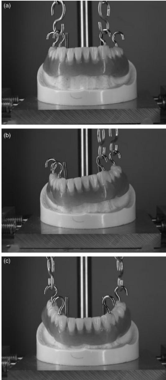
**Fig. 4.** A mandibular-overdenture model permitted evaluation of retention during three types of rotational dislodgements: (a) anterior, (b) lateral and (c) posterior.
