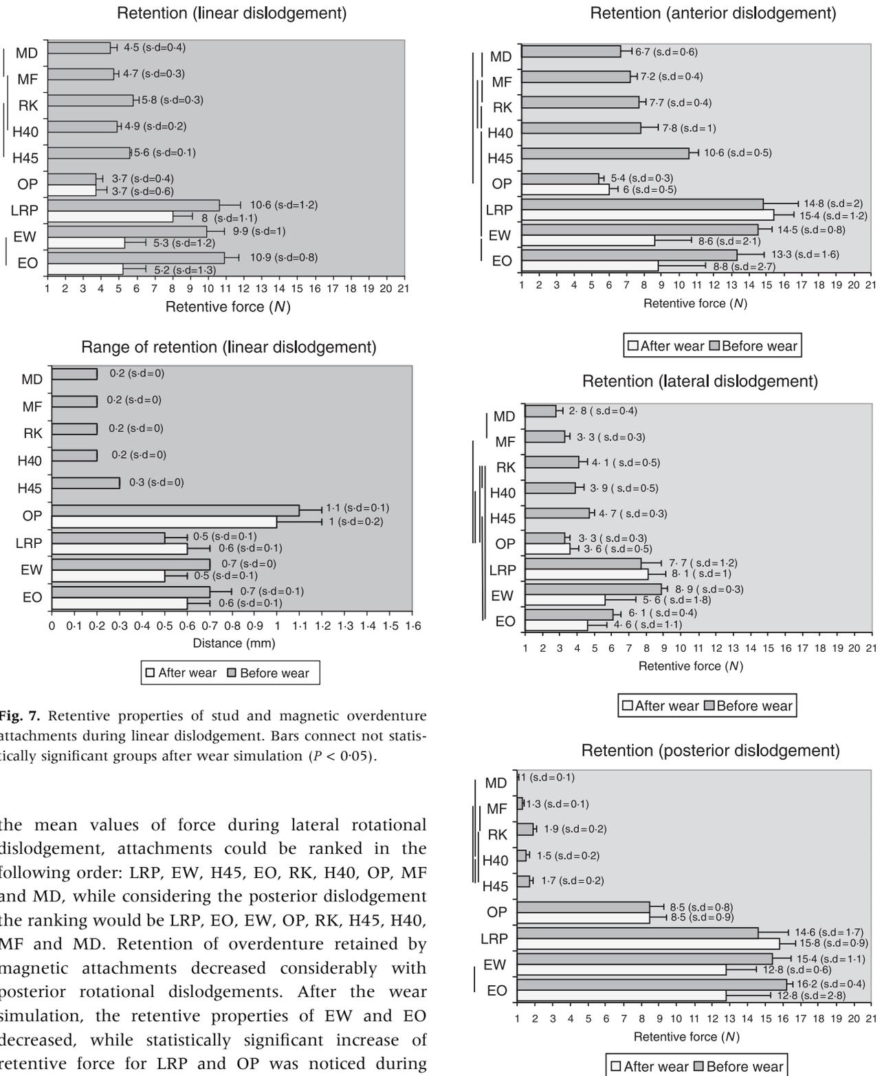
**Fig. 7.** Retentive properties of stud and magnetic overdenture attachments during linear dislodgement. Bars connect not statistically significant groups after wear simulation ( $P < 0.05$ ).
