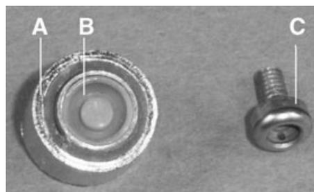
**Fig. 2.** Specimen preparation: (a) metal ring, (b) denture part of an attachment embedded into metal ring by auto-polymerizing resin, (c) tooth (implant) part of an attachment centred on non-ferromagnetic screw.
