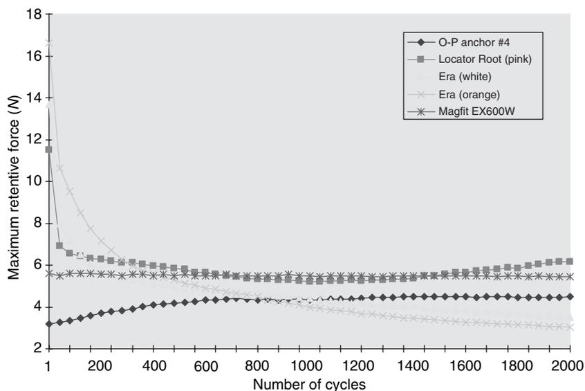
**Fig. 6.** Average curves representing maximum retentive force (N) changes of OP, LRP, EW, EO and MF during consecutive loading (0–2000 cycles).
