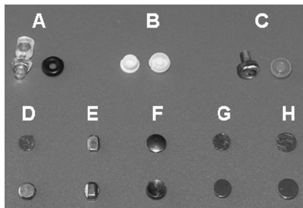
**Fig. 1.** Types of overdenture attachments tested: (a) OP anchor4, (b) ERA overdenture, (c) Locator root, (d) Magnedisc 500, (e) Magfit EX 600W, (f) Magfit-RK, (g) Hyperslim 4013 and (h) Hyperslim 4513.
